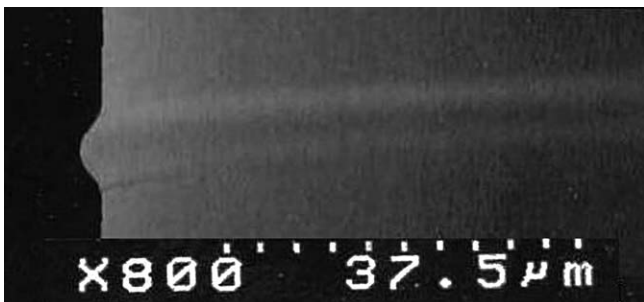
Fig. 6. SEM photograph of a \text{CaF}_2 single mode resonator. Light guiding ridge protrudes only about 2.5 \mu\text{m} above the cylinder.
